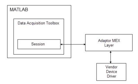
Hardware drivers are provided by the device vendor. For example, to acquire data using a National Instruments<sup>®</sup> board, the appropriate version of the driver must be installed on your system. Hardware drivers are not installed as part of the toolbox, but a suitable driver is usually installed on PCs that are equipped with a sound card. For any other devices, the drivers must be installed.
